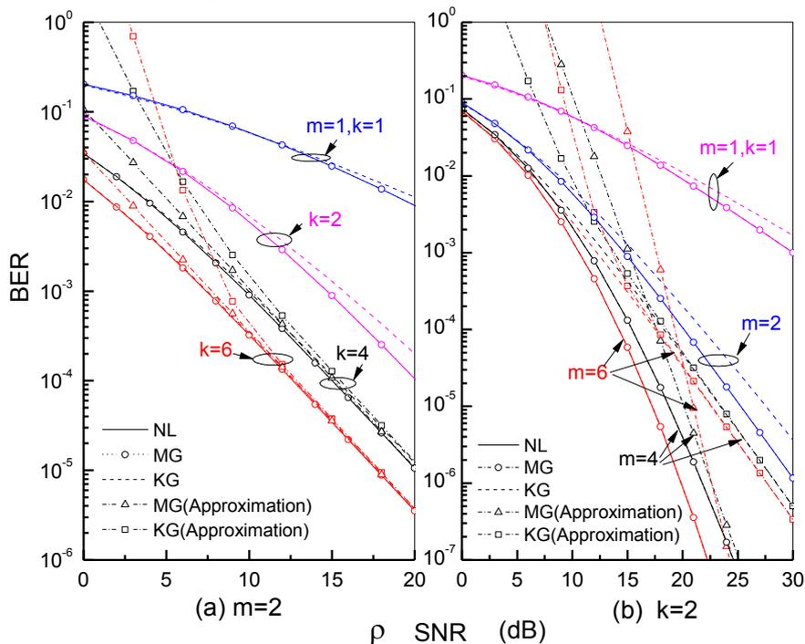
FIGURE 1 Average BER of BPSK for the single-hop link versus un-faded SNR (ρ)
