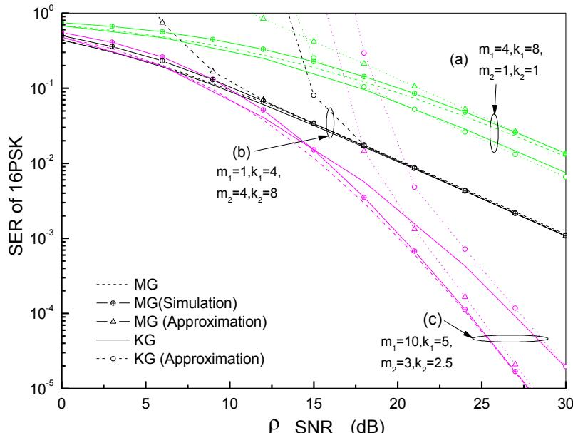
FIGURE 3 Average SER of 16PSK for the dual-hop link versus unfaded SNR ( $\rho$ ) over non-i.i.d fading channels
