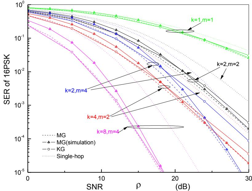
FIGURE 2 Average SER of 16PSK for the dual-hop link versus unfaded SNR ( $\rho$ ) over i.i.d fading channels
