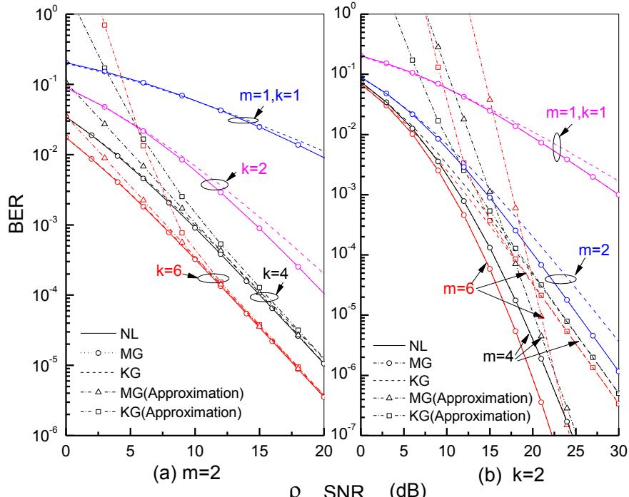
FIGURE 1 Average BER of BPSK for the single-hop link versus un-faded SNR ( $\rho$ )
