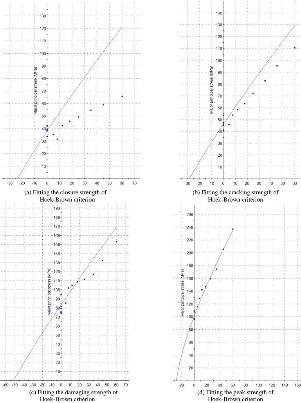
FIGURE 6 Fitting the characteristic strength of Hoek-Brown criterion
