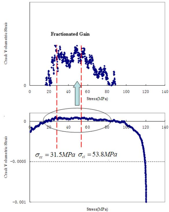
FIGURE 2 The closure stress and cracking stress under D12-28MPa confining pressure
