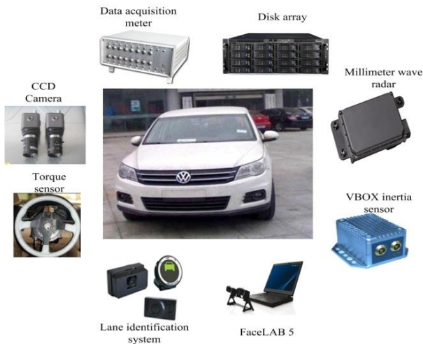
FIGURE 1 Driving behaviour collection platform
