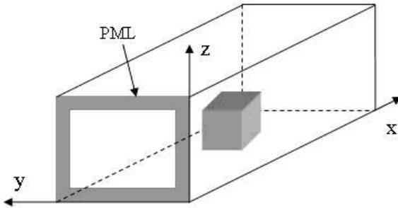
FIGURE 1 Integration domain with PML absorbing boundary condition
